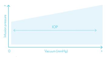
Infusion pressure increases as vacuum increases to smooth out IOP fluctuations.
