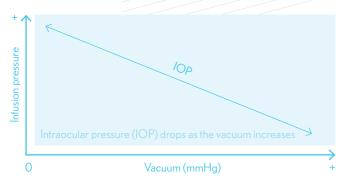
With traditionally fixed infusion pressure, Intra Ocular Pressure (IOP) starts high and then drops as vacuum increases.
